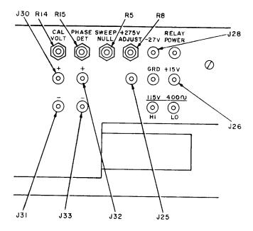
Figure 1. Electronic equipment maintenance kit MK-744/APN-158 - test point and adjustment locations
